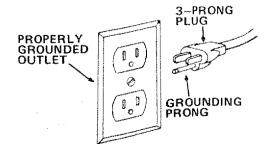
This power tool is equipped with a 3-conductor cord and grounding type plug which has a grounding prong listed by Underwriters' Laboratories Association. The ground conductor has a green jacket and is attached to the tool housing at one end and to the ground prong in the attachment plug at the other end.
